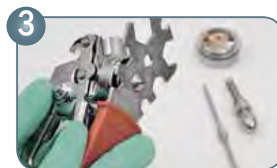
3 And finally, unscrew fluid tip with the ring spanner integrated in the universal spanner.
